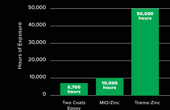
**RIGHT** During salt fog testing (ASTM B 117) Tnemec's zinc-rich primer, Tneme-Zinc, exhibited no blistering, cracking or delaminating after 50,000 hours exposure, with little creepage at the scribe and no more than 1% rusting.
